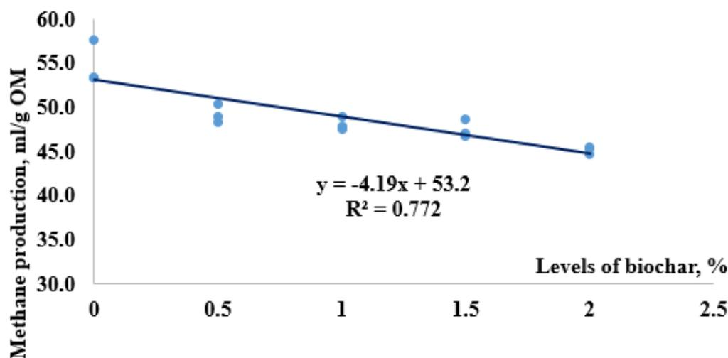
**Fig 3: Linear relationship between biochar (%) and *in vitro* methane production**
